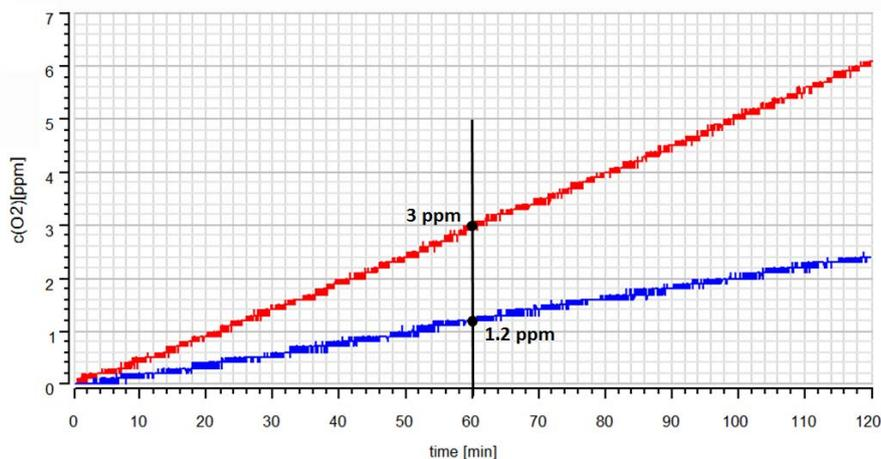
Fig1: Oxygen increase during leak test for Labstar at box internal pressure -10mbar.
