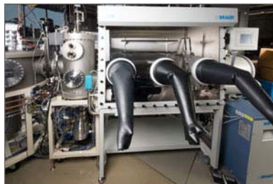
Glove box (right) for loading sources into the thermal evaporator (left) connected to the central vacuum robot (far left) in the Atmospheric Processing platform.
