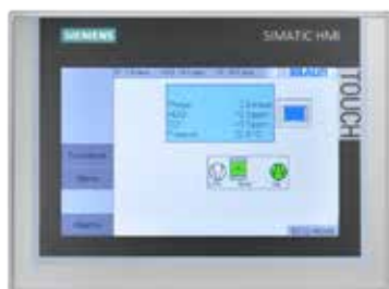
PLC - M. Braun controller with large color touch screen
